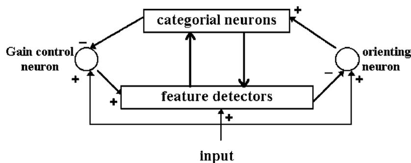
Fig. 4. Basic structure of ART network.
